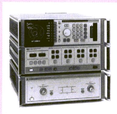
The HP 8510 network analyzer revolutionized the way in which microwave component designers tested their devices.
